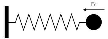
When the ball passes its original equilibrium position, the forces are once again balanced and the restoring force  $F_s$  disappears. However, the ball's momentum carries it past its equilibrium point, compressing the spring and creating a new restoring force in the opposite direction.
