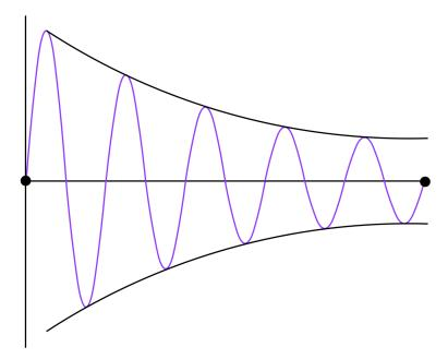
The line connecting the successive crests and troughs of each cycle as it approaches zero is called the wave's decay curve or **envelope**.
