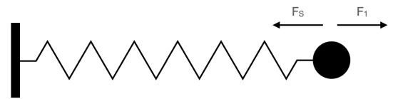
When you release the ball, force  $F_1$  disappears. Since the restoring force  $F_s$  is still present, the ball accelerates in that direction back toward its original equilibrium position.
